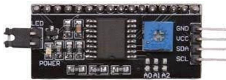
Gambar 7 Modul Inter Integrated Circuit (LCD)
