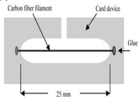
Gambar 3. Spesimen uji tarik standar ASTM D 3379-75
