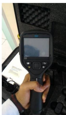
Figure 1. The Thermovision tool type of FIIR E64501 and series 5306A
