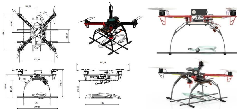
Figure 1. QuadCopter Drone Design
