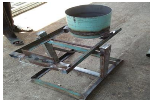
Fig. 4. Big blender frames (in assembling)
