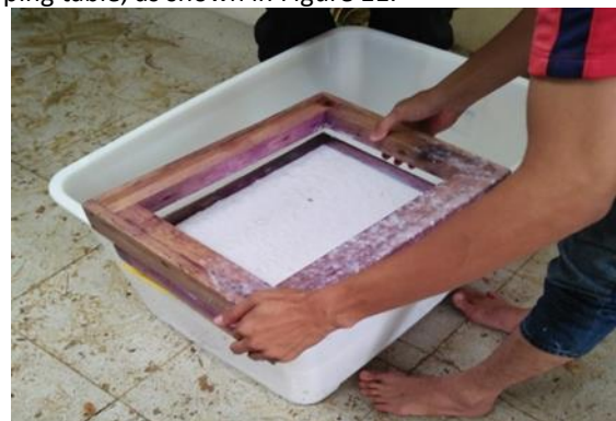
Fig. 9. Screening the pulp paper
