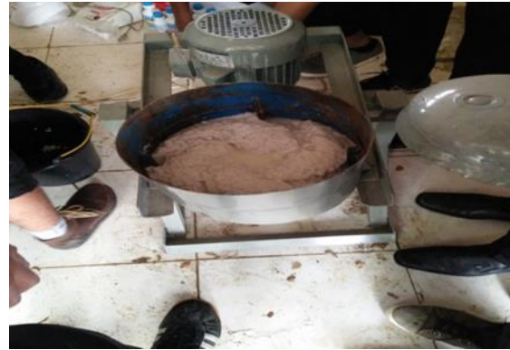
Fig. 7. Pouring pulp into big blender
