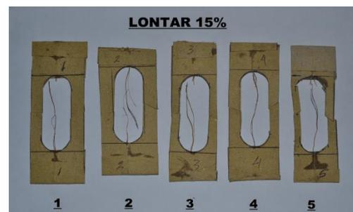
Gambar 3. Spesimen uji tarik standar ASTM D 3379-75
