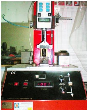
Gambar 1. Alat Uji Tarik Serat *TENSO LAB*
