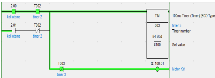
Figure 8. After the time delay is met the induction motor rotates to the left
