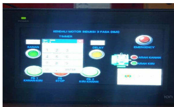
Figure 12. The operator can input the delay time before pressing the pushbutton start on the screen
