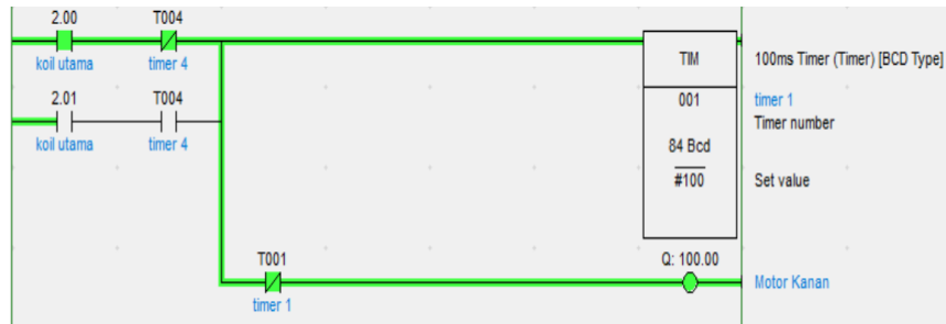
Figure 7. After the time delay is met the induction motor rotates to the right
