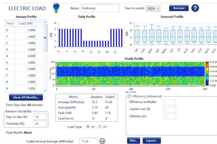
Figure 10. Electrical Load Settings on Homer
