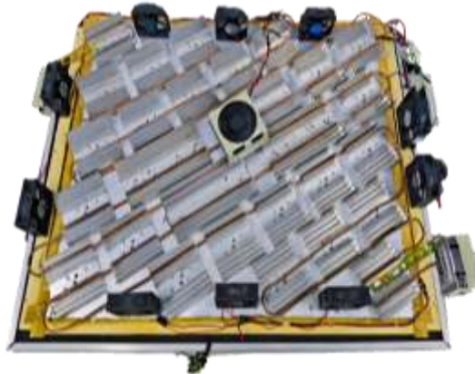
Figure 5. Prototype of the LED cooling system in the solar simulator
