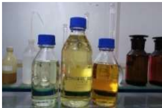
Figure 1. Transformer insulating oil
