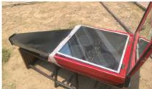
Figure 2. Hybrid box-typesolar cooker (SBC) (Saxena & Agarwal, 2018)
