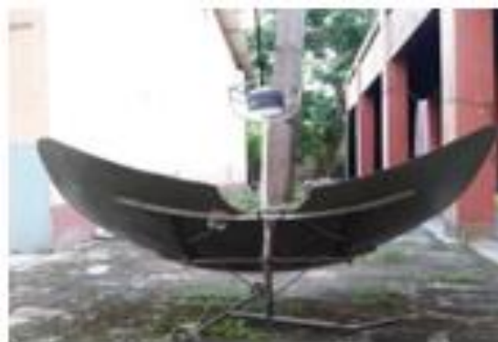
Figure 5. Activated carbon coated aluminum parabolic type domestic solar cooker (Goswami et al., 2019)
