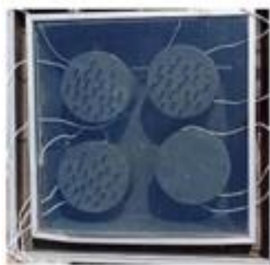
Figure 3. Box-type solar cooker with added aluminum fins (Vengadesan & Senthil, 2021)
