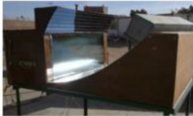
Figure 6. Box-type solar cooker with optogeometric concentrator (Harmim et al., 2012)
