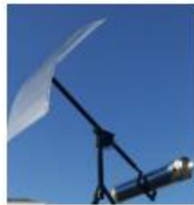
Figure 7. Portable solar cooker using Fresnel lens (Zhao et al., 2018)
