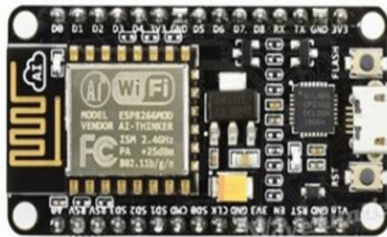
Figure 3. NodeMCU ESP 8266 Wi-Fi device
