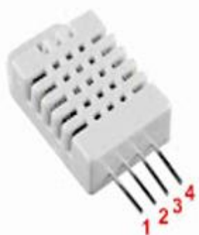
Figure 1. DHT22 components and pin sequence
