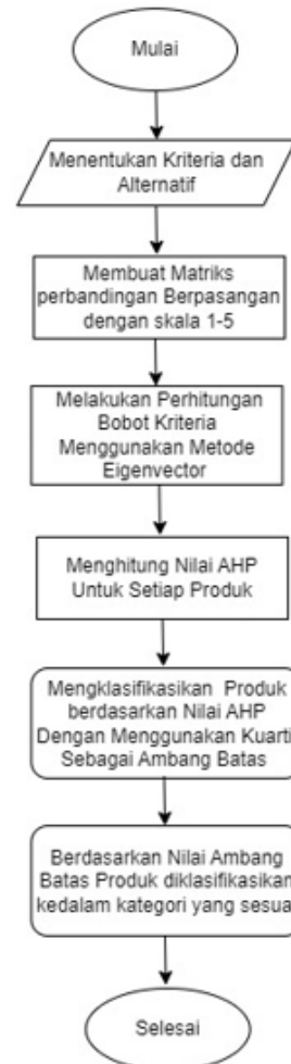
Gambar 2. Skema Metode Analytical Hierarchy Process (AHP)
