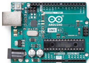
Gambar 2. 6 Arduino Uno R3 [20]
