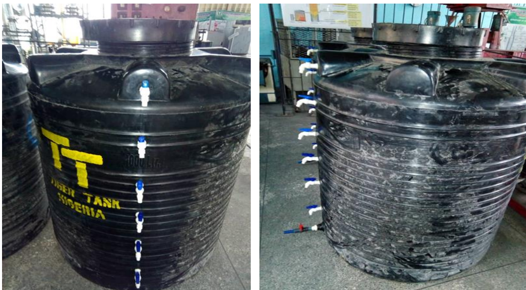
Figure 1. Experimental set-up of cylindrical batch reactor: GP tank with uniformly spaced control valves for collection of samples
