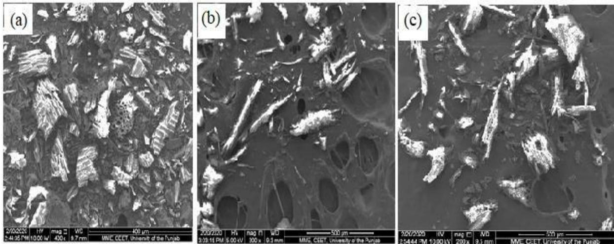
**Figure 14:** SEM Image of (a) AC (b) MSD (c) UMSD
