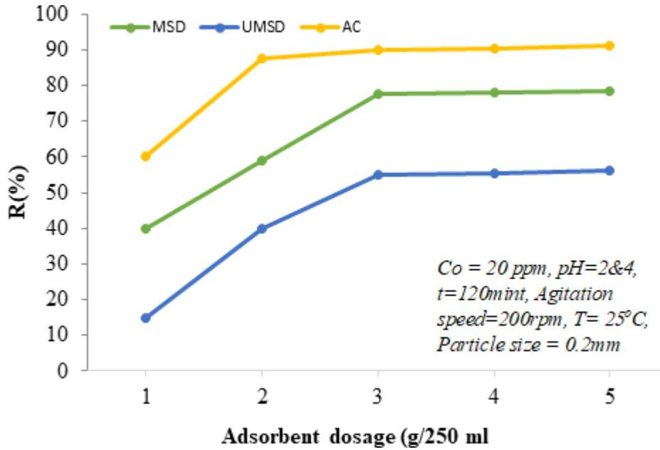
**Figure 5:** Effect of adsorbent dose on the adsorption of Cr (VI) ions
