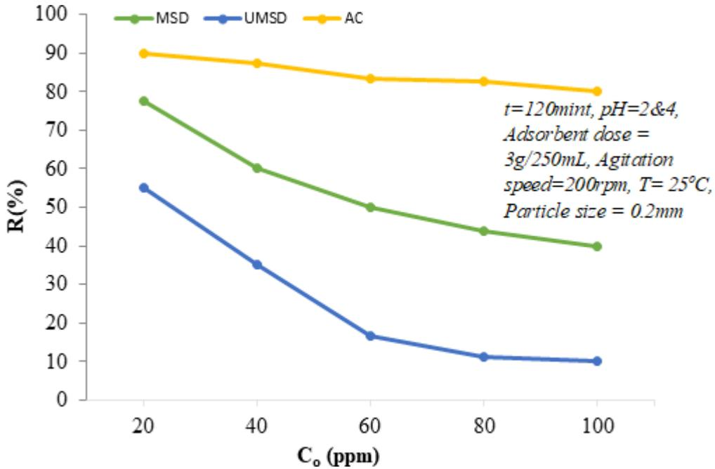
**Figure 6:** Effect of initial concentration of Cr (VI) on the on the adsorption of Cr (VI) ions
