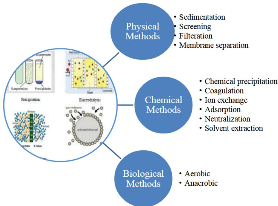
**Figure 1:** HMs removal techniques from wastewater (Stasinakis et al., 2003)
