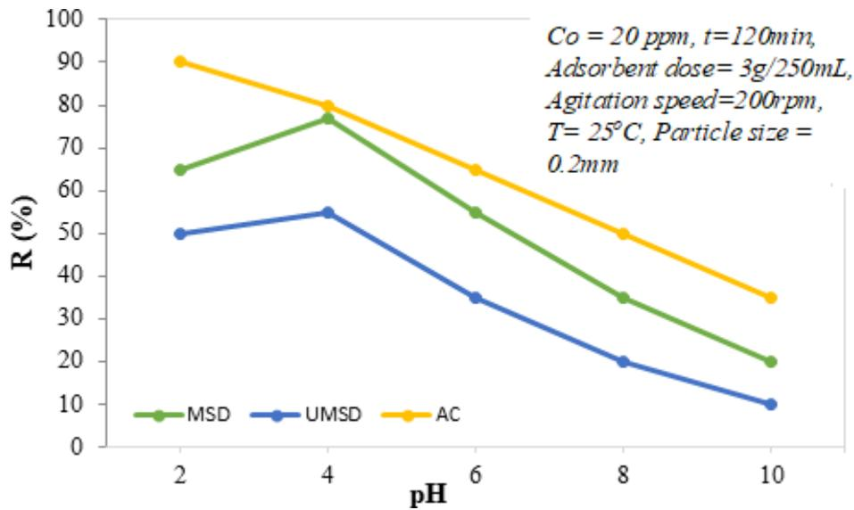
Figure 3: Effect of pH on the adsorption of Cr (VI) ions
