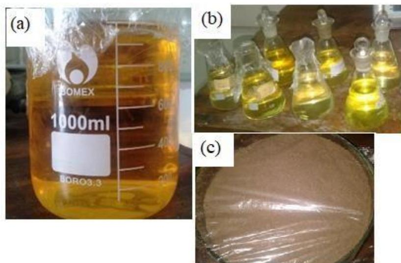
**Figure 2:** (a) Cr (VI) Stock Solution (b) Samples of Cr (VI) Solution with Various Concentrations (c) Modified Mixed Sawdust
