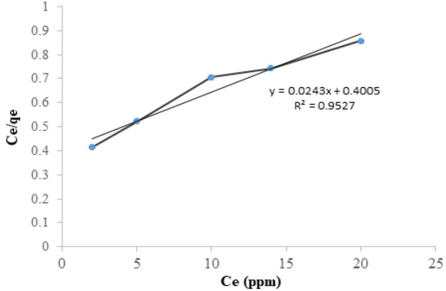
**Figure 9:** Langmuir isotherm in the case of AC
