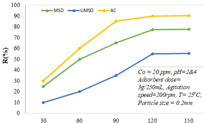
**Figure 4:** Effect of Contact Time on the adsorption of Cr (VI) ions
