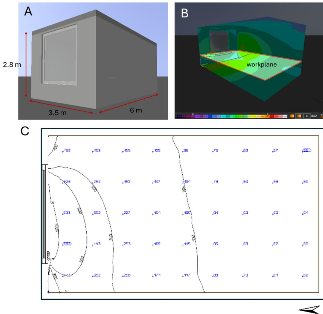
Figure 1. The model of the building created in DIALux Evo (a), the luminance on workplane (b), and the position of the sensor (c).
