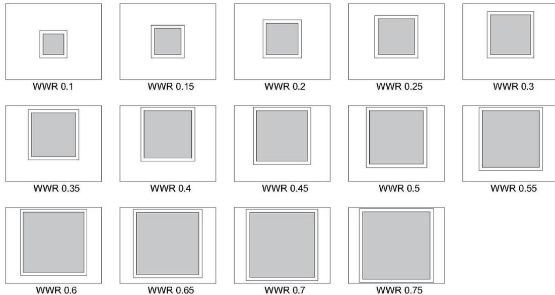
Figure 2. The elevation views of model with different WWR.
