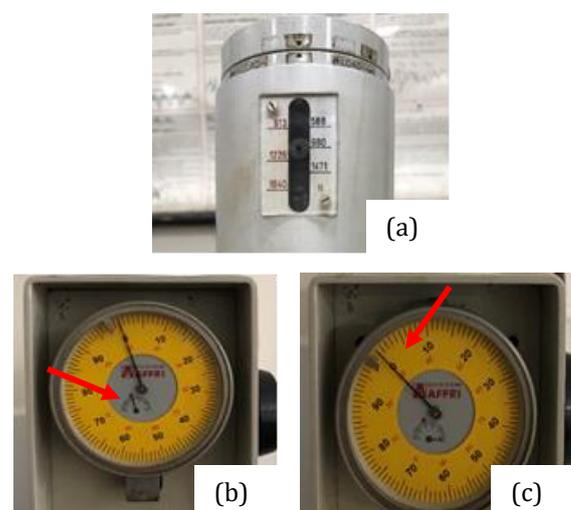
**Figure 1.** (a) Major weight, (b) Giving minor loads, (c) Sets the indicator needle at zero point.
