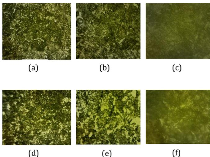
**Figure 5.** AISI 1045 steel raw material microstructure (a)(b)(c). AISI 1020 steel raw material microstructure (d)(e)(f).
