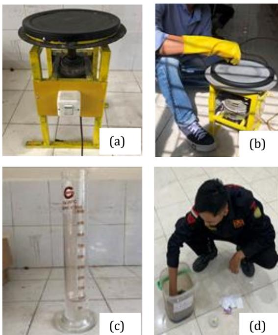
**Figure 2.** Microstructure observation, (a) Grinding polish, (b) Specimen polishing process, (c) The process of preparing the etching material, (d) The process of etching the specimen.
