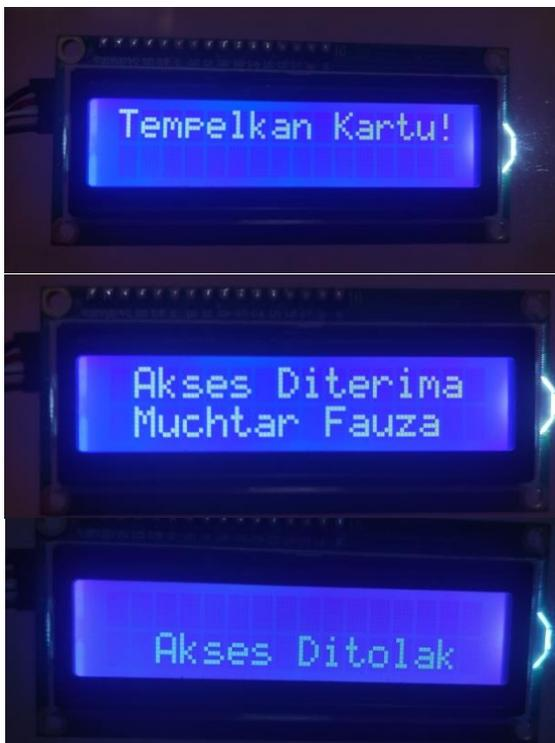
Gambar 19. Hasil Pengujian Liquid Crystal Display (LCD)
