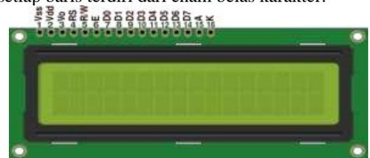
Gambar 5. Liquid cristal display (LCD) 16x2
