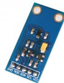
Gambar 2. 9 Modul Sensor Cahaya BH1750
